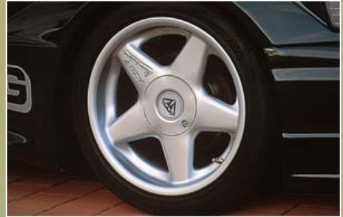
AZEV C front: 8,5Jx17 offset 15 with 235/40-17 rear: 10Jx17 offset 15 with 275/35-17 incl. 15 mm spacers rear
